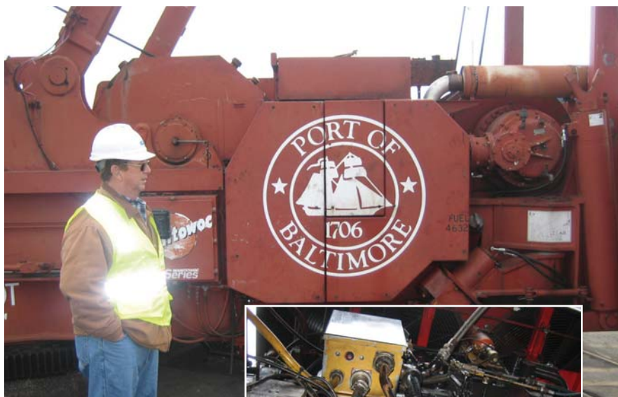
The MPA's "Big Red" crane has a repowered engine that significantly reduces smog-creating emissions.
